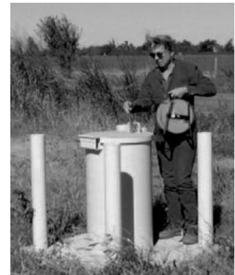
Groundwater Observation Well
